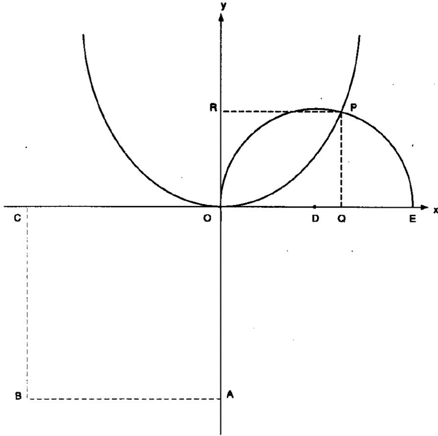
Figure 4: Omar's method of solving the cubic equation  $x^3 + 4x - 8 = 0$ ; the segment  $OQ$  gives the positive root. See text for the method of construction of the square  $ABCD$  to the semi-circle and the parabola. The solution to the cubic is the length  $OQ$ .
