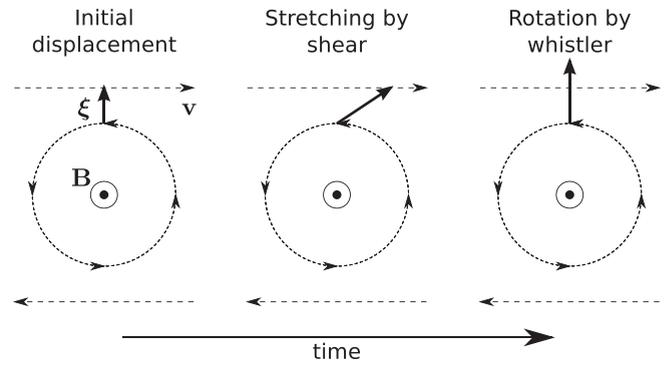
FIG. 1. Cartoon of the density-shear instability. The displacement vector  $\xi$  is stretched by the electron velocity  $\mathbf{v}$  and rotated about the direction of the magnetic field  $\mathbf{B}$ . As a result the initial perturbation is amplified.
