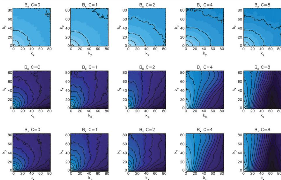
**Figure 5.** Two-dimensional Fourier power spectra at  $t = 0.2$  for 3D EMHD turbulence in the presence of a background field. We show three 2D Fourier power spectra slices of the  $B_x$  datacube, at  $k_x = 1$  (top row),  $k_y = 1$  (middle row) and  $k_z = 1$  (bottom row). Across the columns we show the power spectra for  $C = 0, 1, 2, 4$  and  $8$  (a colour version of this figure is available online at [www.journals.cambridge.org/pla](http://www.journals.cambridge.org/pla)).
