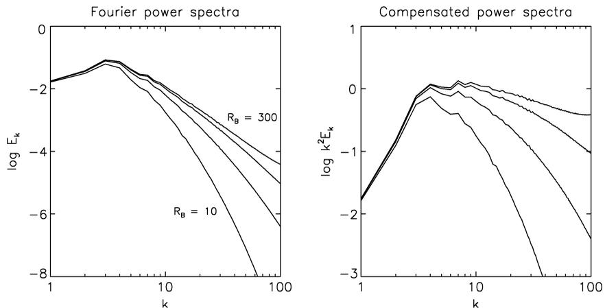
**Figure 1.** Energy spectra of homogeneous 3D EMHD turbulence at  $t = 0.2$ . On the left are shown spectra for  $R_B = 10, 30, 100$  and  $300$ . On the right, compensated spectra  $k^2 E_k$  for the same range of  $R_B$ .
