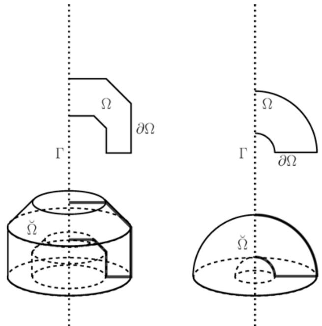
**Figure 1.** The approach we describe aims primarily at solving the Navier–Stokes equation in spherical/spheroidal shells (right). Its flexibility allows, however, to handle axisymmetric containers of more complicated shape (left) that one could use in a laboratory experiment. In each case, the 3-D domain  $\check{\Omega}$  follows from the revolution of its meridional section  $\Omega$  around its axis of symmetry  $\Gamma$ .  $\partial\Omega$  is the boundary of  $\Omega$ .
