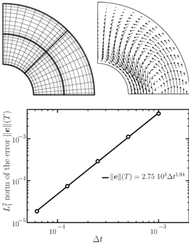
**Figure 5.** Top, SEM mesh (left) with  $n_e = 4$  spectral elements of order  $N = 11$  used for the unsteady Stokes problem (see the text) together with snapshot (right) of harmonic degree 1 velocity field. Bottom, log–log variation of relative error  $\|e\|(T)$  versus time step size for five different values of  $\Delta t$  (white circles). The black fit line corresponds to an exponent of 1.94, which is close to the expected theoretical value (2) for a second-order accurate time-scheme.
