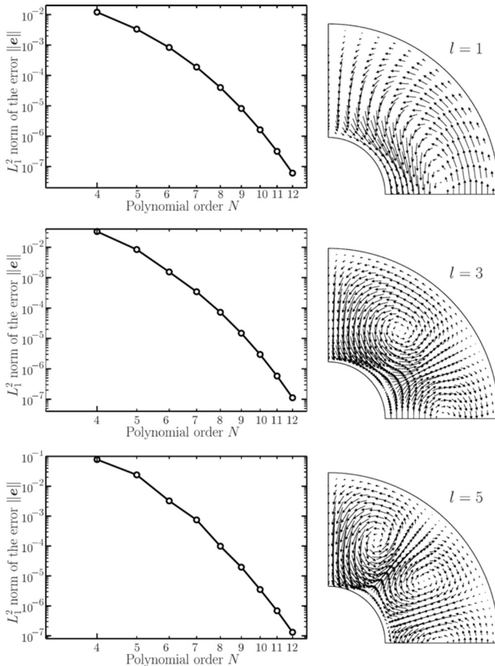
**Figure 4.** Left, log–log plot of relative error (in an  $L_1^2$  sense) for the steady Stokes problem (see the text) as function of polynomial order  $N$  for harmonic degrees  $l = 1, 3$  and  $5$  (top to bottom). Note spectral convergence as  $N$  increases. Right, SEM solution  $\mathbf{u}_h$  for the same harmonic degrees obtained using  $N = 11$ . The analytic reference solution is not shown here, at it is indistinguishable from the SEM solution.
