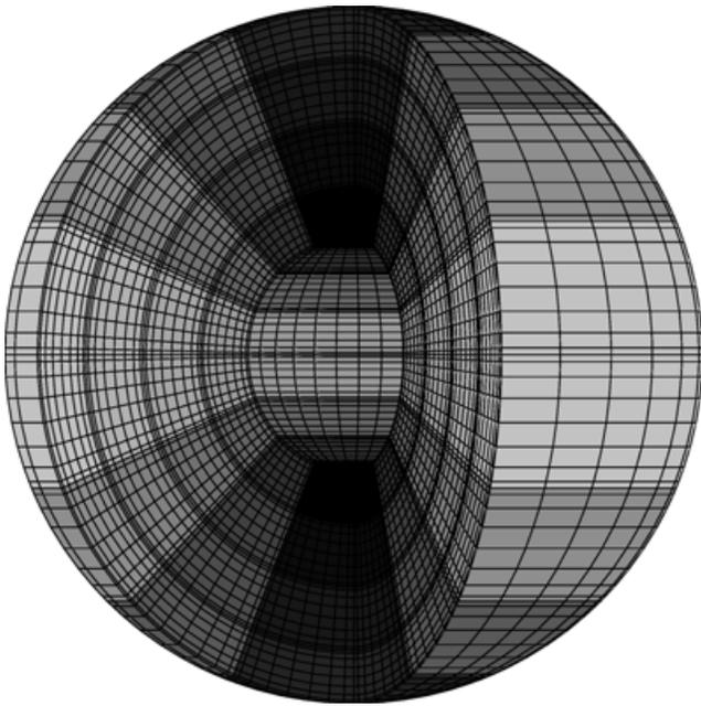
**Figure 9.** 3-D spherical mesh for mixed Fourier–spectral-element approach (see the text). The mesh consists of 32 spectral elements in the meridional plane together with 32 equally spaced points in longitude. The spatial domain decomposition (indicated by grey-scale) for parallel processing is illustrated for 16 processors handling two spectral elements each.
