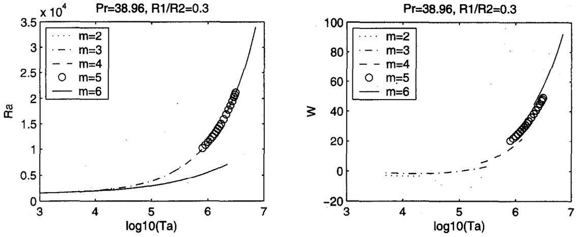
Fig. 5. a - Stability curve: critical Rayleigh number as function of  $Ta$ ; b - Drift velocity as function of  $Ta$
