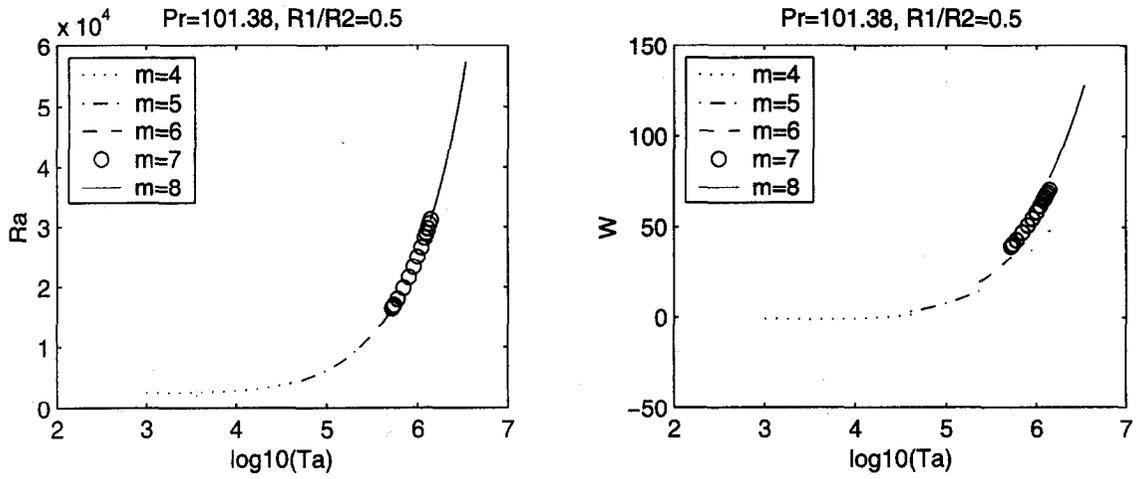
Fig. 6. a - Stability curve: critical Rayleigh number as function of  $Ta$ ; b - Drift velocity as function of  $Ta$
