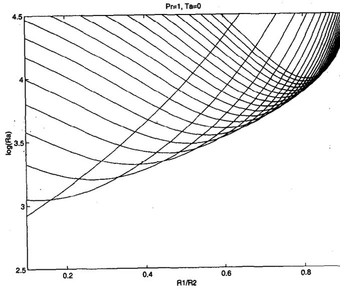
Fig. 2. Stability curve: critical Rayleigh number as function of  $\eta$ , for  $l = 1$  to 20, increasing from left to right.
