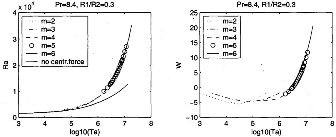
Fig. 4. a - Stability curve: critical Rayleigh number as function of  $Ta$ ; b - Drift velocity as function of  $Ta$
