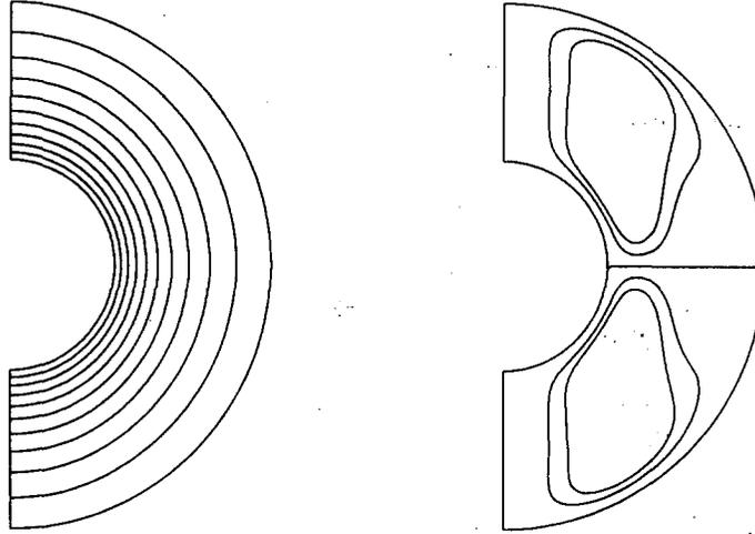
Fig. 1. The basic state for  $Ta > 0$ : left - Temperaturefield , right - streamfunction (equatorsymmetrical)
