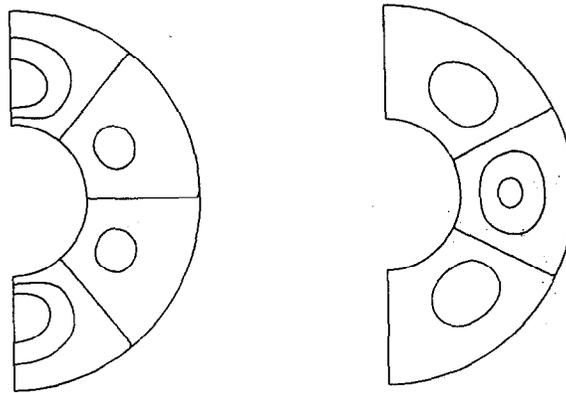
Fig. 3. An example of the perturbation solution, with the temperature on the left, and the meridional circulation on the right. This particular solution corresponds to  $Pr = 1$ ,  $\eta = 0.4$ ,  $l = 3$
