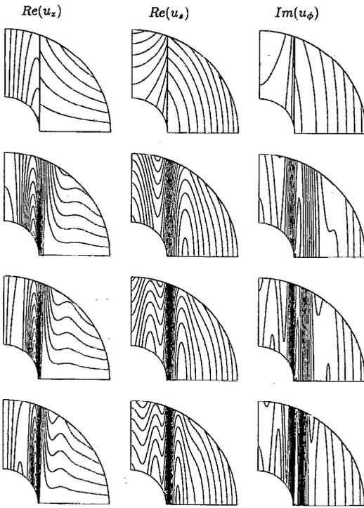
FIG. 1. At the top, the inviscid solution (12) corresponding to  $\mathbf{f}_0$ . Below, the viscous solutions at  $\epsilon=10^{-4}$ ,  $10^{-4.5}$ , and  $10^{-5}$ . From left to right, the real parts of  $u_z$  and  $u_s$ , and the imaginary part of  $u_\phi$ . Contour intervals of 0.2 for  $u_z$ , 0.4 for  $u_s$ , and 2 for  $u_\phi$ .
