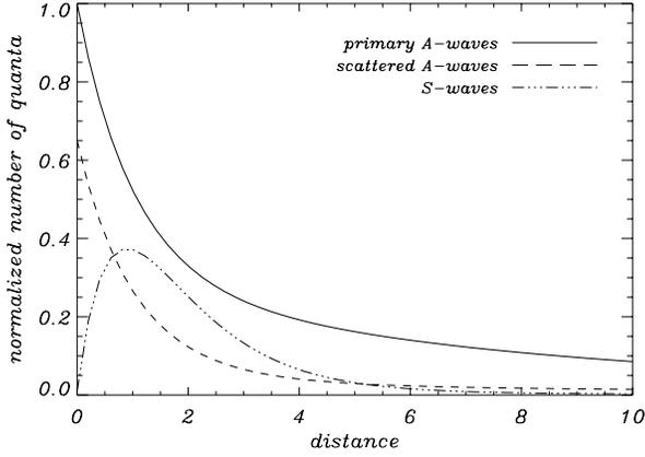
**Fig. 3.** Solutions of the backscattering system. By order of decreasing line thickness we show  $N_+/N_+(0)$ ,  $N_-/N_+(0)$  and  $N_s/N_+(0)$ . The distance unit is the scattering length defined by  $V_*/\omega N_+(0)$ . In this example  $\gamma_+ = 0.1$ ,  $\gamma_- = 0.05$  and  $\gamma_s = 0.69$ .
