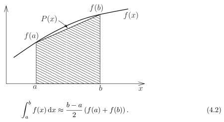
Thus, the trapezium rule can be obtained by integrating the linear interpolation function
