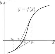
Suppose we have an initial guess  $p_o$  where f and f' are known. Then,  $p_1$ , the intersection of the x-axis with the tangent to f in  $p_0$ , is an improved estimate of the root.
