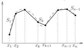
The coefficients  $a_k$  and  $b_k$  are determined by the conditions (i)  $S_k(x_k) = f_k$  and (ii)  $S_k(x_{k+1}) = f_{k+1}$ , k = 1, ..., n-1. Thus,
