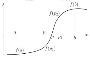
Bisection gives a simple and robust method for bracketing the root p. The algorithm works as follows:
