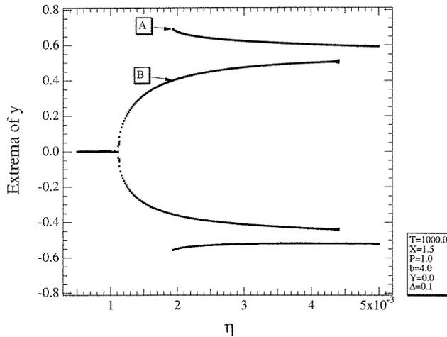
**Figure 3.** Bifurcation diagram of the extrema of the deviation of the field from steady state as a function of injection. The solutions are computed from the rate equations (1) and (2) using the same values of the parameters as in figure 2. The points denoted by A and B indicate where the spectra in figures 2(a) and (b) were computed numerically.
