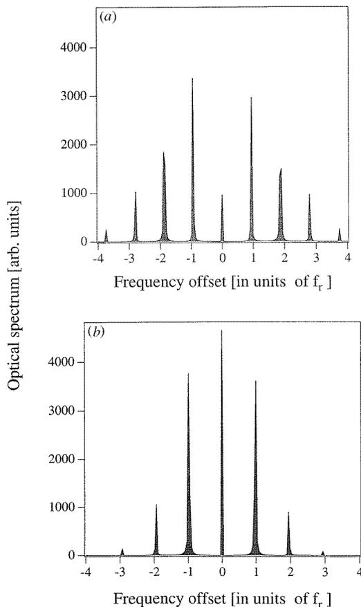
**Figure 2.** Numerically computed optical spectra from the single-mode rate equations (1) and (2) for  $T = 1000$ ,  $b = 4$ ,  $P = 1.0$ ,  $\eta = 0.002$  and  $\Omega/\omega = 0.1$ . The zero of the frequency scale denotes the frequency of the master laser.
