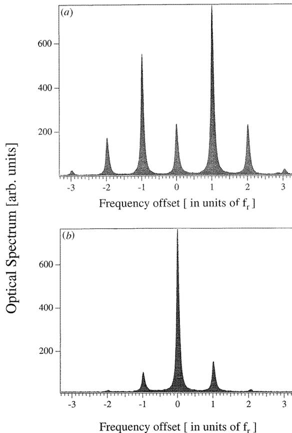
**Figure 1.** Experimentally obtained optical spectra of the laser subject to injection in the neighbourhood of the Hopf bifurcation.  $f_r$  is defined as the free-running relaxation oscillation frequency,  $f_r = (1/2\pi)\sqrt{2P/T}$ .
