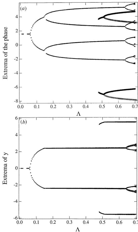
**Figure 5.** Bifurcation diagram obtained numerically from the phase equation (8) for  $T = 1000$ ,  $b = 10$ ,  $P = 0.5$  and zero detuning. (a) Shows the extrema of the phase  $\Phi$  versus injection  $\Delta$ . (b) Shows the extrema of the field versus injection.
