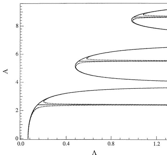
**Figure 4.** Bifurcation diagram of the amplitude  $A$  of the periodic solution versus  $\Lambda$  constructed from the analytic solutions of the phase equation for  $T = 1000$ ,  $b = 10$ ,  $P = 0.5$ . Full curves are for  $\Delta = 0$  and dotted curves for  $\Delta = 0.01$ .
